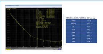
RMS jitter stands at a remarkable 66 fs, while the current consumption remains below 40 mA.
