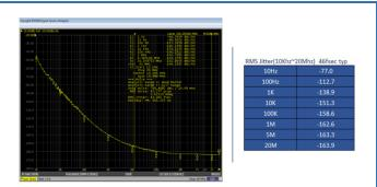
AKER product stands out with an exceptional phase noise rating of 46 fs and an impressively low current consumption of under 40 mA.
