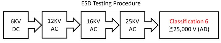
DC=Direct Contact Discharge, AD = Air Discharge
